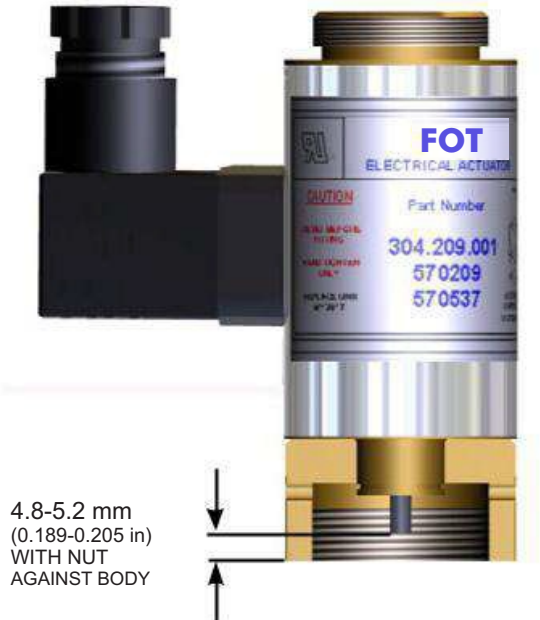
Actuator Non-Fire Position
