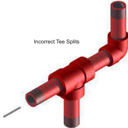
Side tee orientation incorrect"
