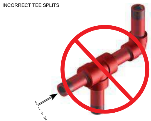
SIDE TEE ORIENTATION "INCORRECT"
