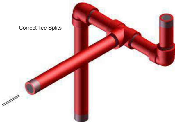
Bull tee orientation "correct"
