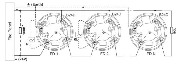
\*ATTENTION: When the EOLmodule is only a capacitor, IT IS OBLIGATORY TO CONNECT a 100K resistor in parallel at the beginning of the line!
