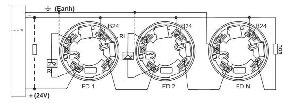
\*ATTENTION: When the EOLmodule is only a capacitor, the line! IT IS OBLIGATORY TO CONNECT a 100K resistor in parallel at the beginning of
