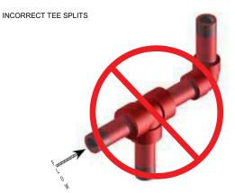
FIGURE 5-5 SIDE TEE ORIENTATION "INCORRECT"
