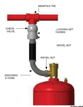
FIGURE 6-4 80 mm (3 IN.) HOSE/CHECK VALVE INSTALLATION: Part No. 300013
