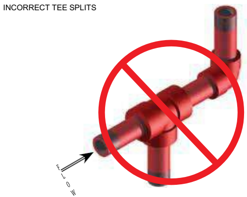
SIDE TEE ORIENTATION "INCORRECT"
