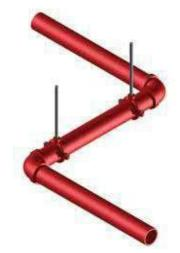
FIGURE 6-6 ELBOW SUPPORT: Part No. 300015
