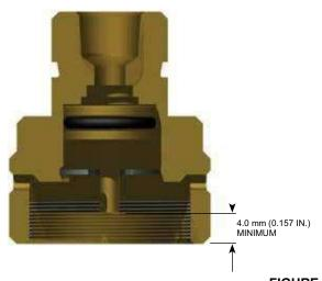
FIGURE 6-9 PNEUMATIC ACTUATOR NON-FIRED POSITION: Part No. 300018
