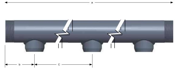
FIGURE 6-3 TYPICAL MANIFOLD ASSEMBLY: Part No. 300012
