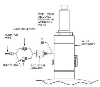
FIGURE 6-12 ACTUATION ISOLATOR INSTALLATION
