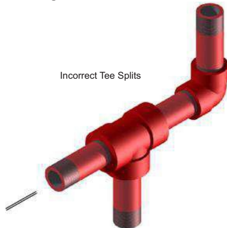
Figure 12 - Side tee orientation "incorrect"
