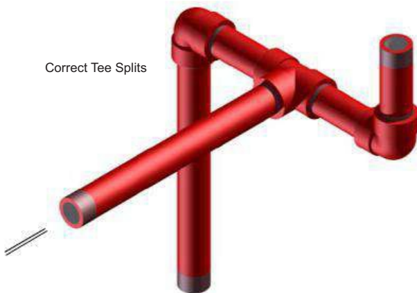
Figure 13 - Bull tee orientation "correct"
