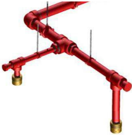
Figure 7 - Typical Manifold System: Part No. 300017
