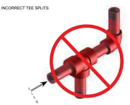
FIGURE 5-5 SIDE TEE ORIENTATION "INCORRECT"
