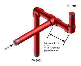
Figure 11 - Side tee orientation "correct
