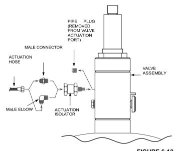
FIGURE 6-12 ACTUATION ISOLATOR INSTALLATION
