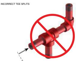
FIGURE 5-5 SIDE TEE ORIENTATION "INCORRECT"
