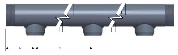
FIGURE 6-3 TYPICAL MANIFOLD ASSEMBLY: Part No. 300012
