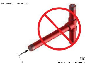
FIGURE 5-7 BULL TEE ORIENTATION "INCORRECT"
