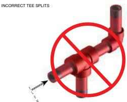
FIGURE 5-5 SIDE TEE ORIENTATION "INCORRECT"
