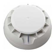
SensoFOT F10 is a fixed temperature detector with digital processing algorithm. The detector is designed to detect temperatures above 60°C (class A2S, according EN54-5). SensoFOT F10 is suitable for installing in any conventional fire alarm system designed with fire alarm panel with fire alarm threshold between 10mA and 15mA.
