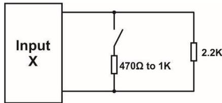
Figure 14 – Connections to the supervised inputs
