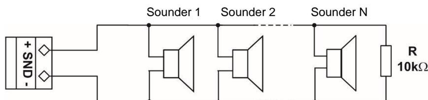
**Figure 13 – Connecting sounders to SND output**
