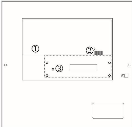
The module is mounted on the back side of the metal cover. The connection is via an interface connector to the indication board of the panel – J1 terminal on the module to the P2 terminal on the panel's indication board. The FOT-IVY ML is fixed to the cover with 5 screws on the location shown on Figure 19.
