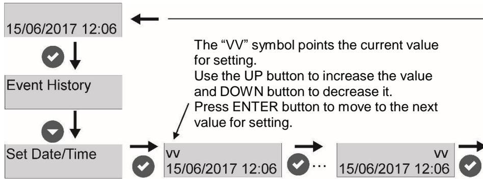
Set in sequence the current date, month and year, and time [Hour:Minutes]. After the last confirmation the module exits to normal operation mode.
