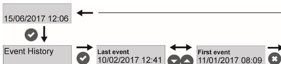
The first message in the list is the last event in the system (the newest recorded in the log). On the second row are viewed the date and time of occurring. To review the second and following messages, press the DOWN arrow button. To turn back, start pressing the UP arrow button. See APPENDIX A for the detailed list of all messages with its description.
