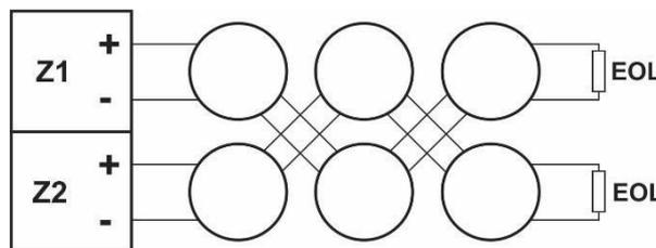
**Figure 11 – Cross-zoning connection diagram for Zone 1 and Zone 2**
