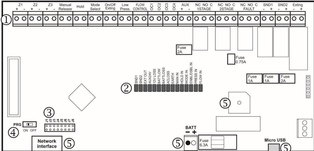
Figure 7 – Main PCB of FOT-IVY control panel
