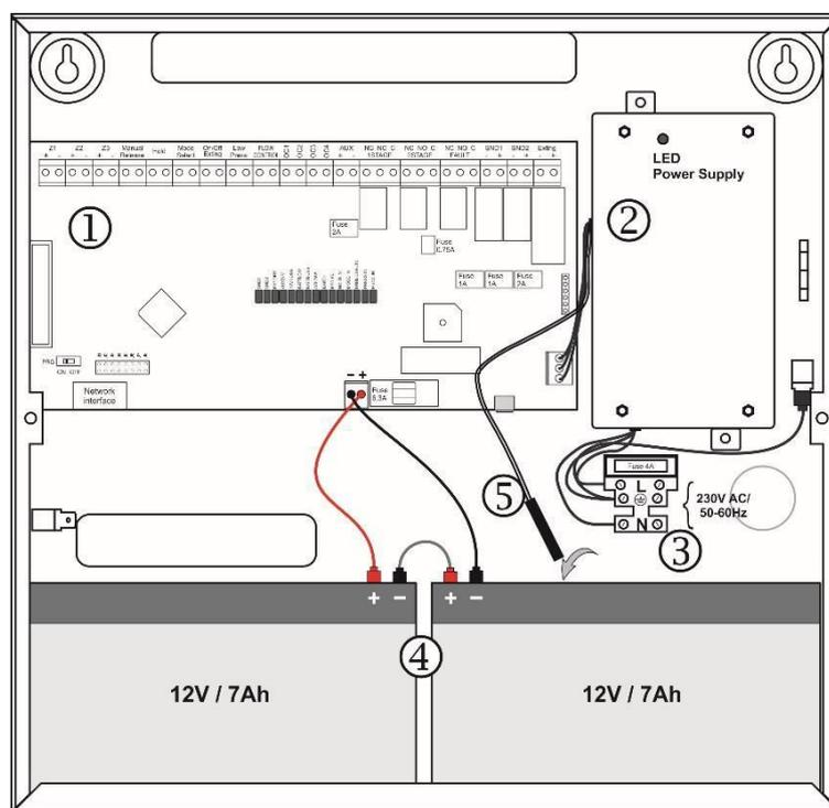
Figure 6 – Configuration of the modules in the box
