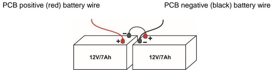
**Figure 10 – Serial connection of the batteries**
