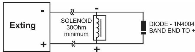
Figure 15 – Example of wiring a solenoid
