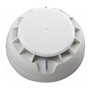
SensoFOT F10 is a fixed temperature detector with digital processing algorithm. The detector is designed to detect temperatures above 60 °C (class A2S, according EN54-5). SensoFOT F10 is suitable for installing in any conventional fire alarm system designed with fire alarm panel with fire alarm threshold between 10mA and 15mA.
