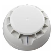
SensoFOT R20 is a rate-of-rise temperature detector with digital processing algorithm. The detector is designed to detect temperatures above 58 °C (class A1R, according EN54-5).
